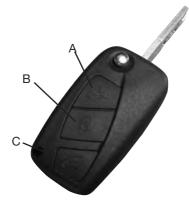
• Pressing button 'A' will unlock the base vehicle cab doors only.
