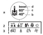
a = Boiler \* - Warm water boiler is switched on.
