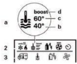
a = Boiler \* - Warm water boiler is switched on. - Warm water temperature 40 °C
