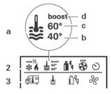
a = Boiler \* - Warm water boiler is switched on.
