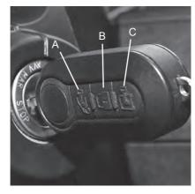
• Pressing button 'A' will unlock the base vehicle cab doors only.
