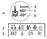
a = Boiler \* - Warm water boiler is switched on.  $b = 40^{\circ}$ - Warm water temperature 40 °C  $c = 60^{\circ}$  Warm water temperature 60 °C d = boost \* - Targeted, fast heating of the content
