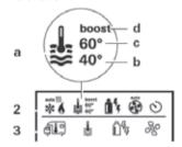
a = Boiler \* – Warm water boiler is switched on. b = 40° – Warm water temperature 40 °C c = 60° – Warm water temperature 60 °C
