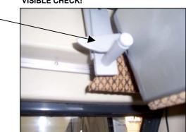
Ensure locking bars are fully latched over the locking pins
