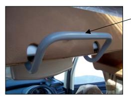
Release securing strap and rotate locking Handle forwards to release locking bars From locking pins
