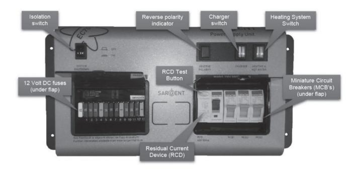
The EC 700 has a shutdown feature that can be used when the vehicle is in storage. This allows the leisure electronics to be turned off when not required to save battery power. When in the 'off' position the alarm and tracking system supplies are still active, all other supplies are turned off.
