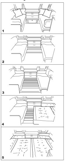
The two single beds can be easily converted into a double bed by pulling out the bed slats, stored beneath the chest of drawers or stored in the bed slat box at the front/end of the caravan. Arrange seat cushions appropriately.
