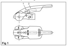
Coupling handle (Fig. 1/Item 1), Stabiliser Lever (Fig. 1/Item 2)
