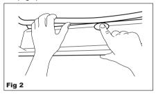
(ii) Whilst depressed, slide the bar to the desired position and locate into the stops provided (Fig 3).
