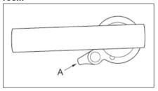
To open the door, push the small lever down (identified in the drawing as A) then to unlock, push this lever back to the original position.
