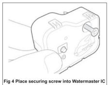
Step 6 - Plug Watermaster IC onto socket (see Fig 5) and tighten screw (NB -Do Not Overtighten)
