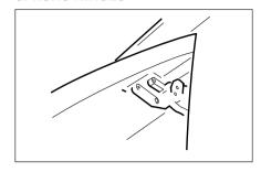
Overhead lockers will use sprung hinges. These are suitably strong enough when closed to securely retain the door and prevent it from opening in transit. Pulling the handle towards you with moderate force is sufficient to open the locker door and hold it in the open position.
