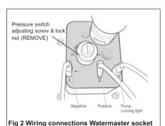
Step 3 - Unscrew and remove the pressure switch adjusting screw and locking
