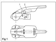
Coupling handle (Fig. 1/Item 1), Stabiliser Lever (Fig. 1/Item 2)
