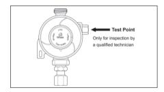
Your new Elddis caravan has been fitted with a fully approved gas regulator designed to operate at a gas pressure of 30Mbar. Your regulator is fitted with a test point, which is accessed via the inlet at the side of the regulator. This access point is only for carrying out gas pressure tests and should not be used for any other purpose.
