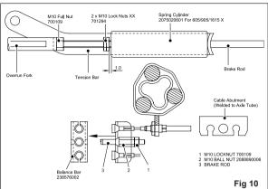
give 1mm of clearance on the spring cylinder. This cylinder (the energy store for the handbrake operation) must be able to rotate only, not slide on the brake rod.
