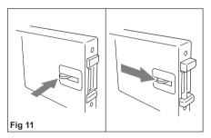
If the refrigerator is taken out of service for an extended period, close the isolation tap and the gas cylinder valve.
