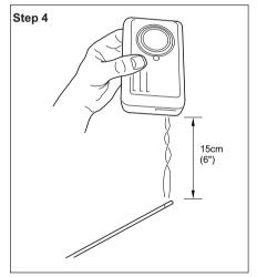
Turn the detector on its side so that the vents on the right hand side of the detector are pointing downwards. Hold the burning incense stick around 15cm (6 inches) below the detector, so that the smoke enters the vents on the side of the detector. An increase in the localised carbon monoxide level within the sensor to more than 50ppm will cause the sounder to sound for one cycle of
