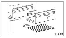
Unlock the freezer compartment on both sides (1)
