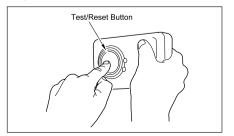
Cover the sounder vents with one hand. Press and hold the Test/Reset button down with your thumb/finger until the Power LED illuminates green and the sounder sounds for a second time (this should happen after around 5 seconds). Release the Test/Reset button. Upon releasing the Test/Reset button the Power LED will flash green once every second. This indicates that the sampling rate of the detector has increased and can be tested using a known source of CO.
