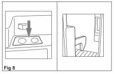
Shut the door again by pushing it to close. The snapping into the lock can be heard. **Note:** If the vehicle is stationary for a long period, the locking hook may be clamped by means of a lockbar. The door may now be opened by just pulling it without need of pressing the locking button. See below.
