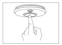
• The unit will give an audible alarm consisting of 2 cycles of 3 loud beeps, then stop automatically.
