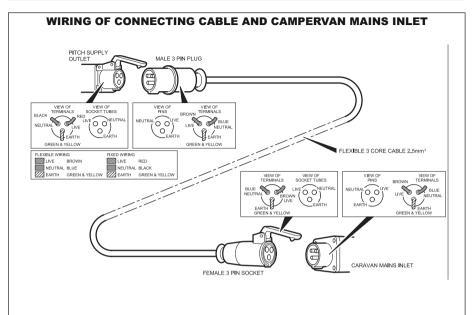
WARNING: It is essential that connections are made exactly as shown. If terminal markings are not in accordance with the above diagram they must be ignored.
