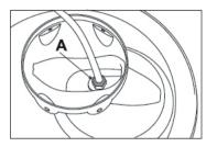
Loosen the nut (A) slightly (by one quarter of a turn).
