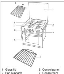
The types of burners may vary depending on the type of appliance. Refer to Technical specifications for further details.
