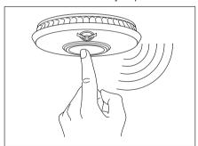
Your alarm will silence and enter into a reduced sensitivity reset cycle for approximately 10 minutes.
