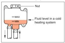
**CAUTION:** The heating system comes installed with glycol heating fluid. If the fluid level is too low you must fill the system to the right level before operating the heating system.
