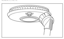
WARNING: Your smoke alarm may false alarm when it is being cleaned using a vacuum cleaner.
