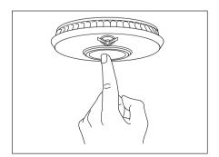
The unit will give an audible alarm consisting of 2 cycles of 3 loud beeps, then stop automatically.
