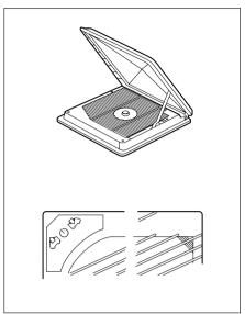
The Omnivent is a double-glazed roof light constructed from a synthetic ultra-violet screened material. Its side-operating mechanism allows a completely free central opening with built-in fixed ventilation when closed. It operates as an extractor fan and air intake fan.
