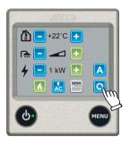
The control panel showing the settings menu. Press the tool symbol to access the tools menu.
