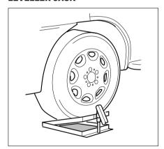
Place the leveller jack, folded flat, in front of the wheel that is to be raised to level the axle. Drive the motorhome onto the leveler jack and adjust the height until the spirit level shows that the motorhome is laterally level.
