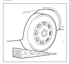
Reverse onto your pitch about a foot further back than you wish to end up. Then place the levelling ramp in front of the wheel that needs to be raised.
